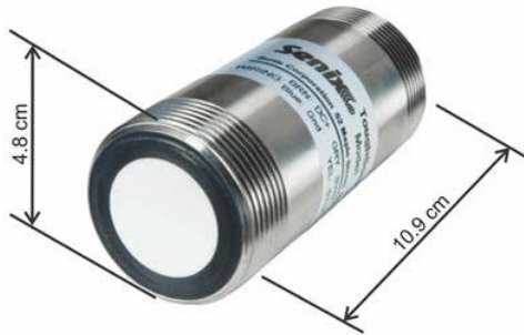
FIGURE 9. Photograph of a Senix ToughSonic 30 ultrasonic distance module used in some of the BMRSS units. It has a range of up to 9.1 m (30"). In most locations, we use the ToughSonic 50, which has a 15.2 m range (50").
