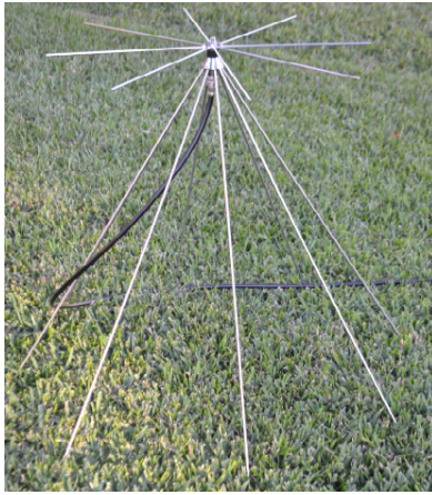
FIGURE 3. The Diamond D-130NJ antenna is a wideband discone antenna that has a nominal gain of 2 dBi and an operating bandwidth of 25 MHz to 1300 MHz.
