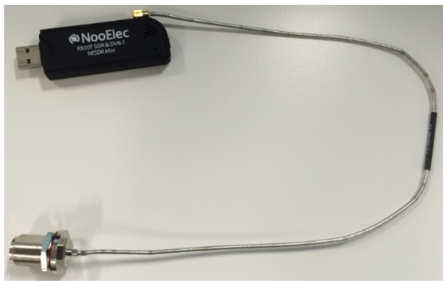
FIGURE 4. The RTL-SDR is connected to the Pasternack PE-SR405FL RF cable, which is used to interface the LMR-400 RF cable to the MCX connector on the RTL-SDR.
