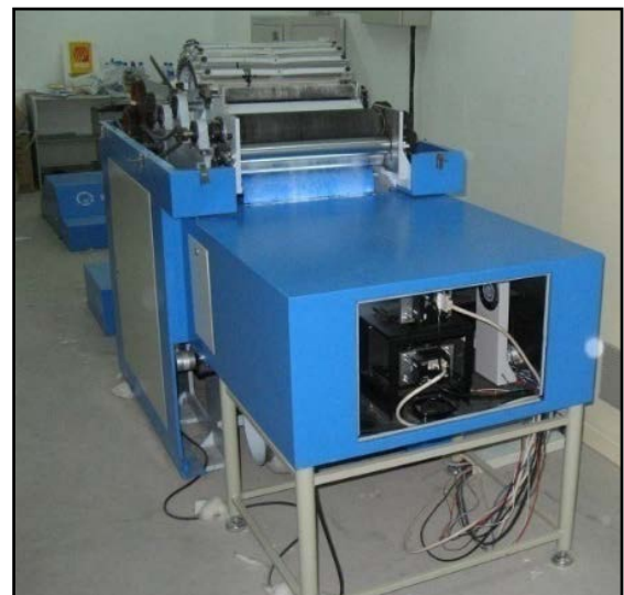
FIGURE 2. Foreign fiber image acquisition system.
