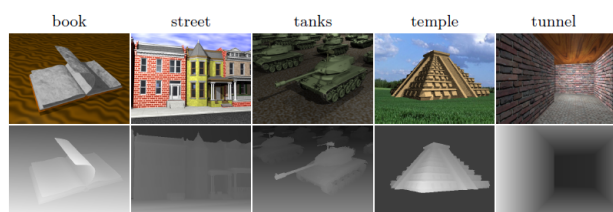
FIGURE 7. Selected frames and disparity maps from synthetic stereo video sequences.
