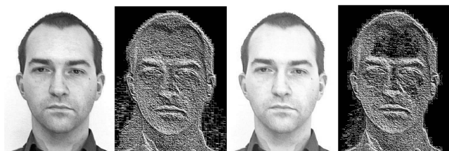
FIGURE 5. Comparison of high lightness variation in face images using the LBPH algorithm.
