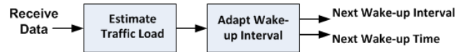
FIGURE 3. Traffic-aware dynamic MAC protocol consists of two components (i.e., traffic estimation and adaptive wake-up interval algorithm).
