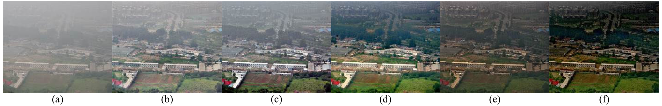
FIGURE 11. Results of some defogging algorithms on an aerial photo without a sky area. (a) original image. (b) CLAHE [108]. (c) MSRCR [98]. (d) Tarel and Hautiere [19]. (e) Meng et al. [81]. (f) Nishino et al. [82].
