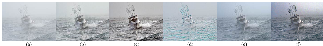
FIGURE 15. Results of some defogging algorithms on a sea scene with thin fog. (a) original image. (b) CLAHE [108]. (c) MSRCR [98]. (d) Tarel and Hautiere [19]. (e) He et al. [29]. (f) Meng et al. [81].
