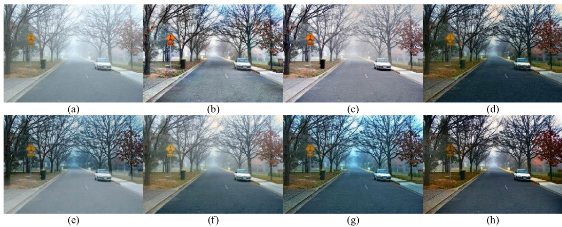
FIGURE 8. Comparisons of some classical defogging algorithms with a road scene. (a) original image. (b) CLAHE [108]. (c) MSRCR [98]. (d) Fattal [48]. (e) Tarel and Hautiere [19]. (f) He et al. [29]. (g) Meng et al. [81]. (h) Ancuti et al. [31].
