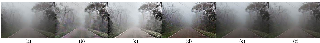
FIGURE 13. Results of some defogging algorithms on a road scene with dense fog. (a) original image. (b) CLAHE [108]. (c) MSRCR [98]. (d) Tarel and Hautiere [19]. (e) He et al. [29]. (f) Meng et al. [81].
