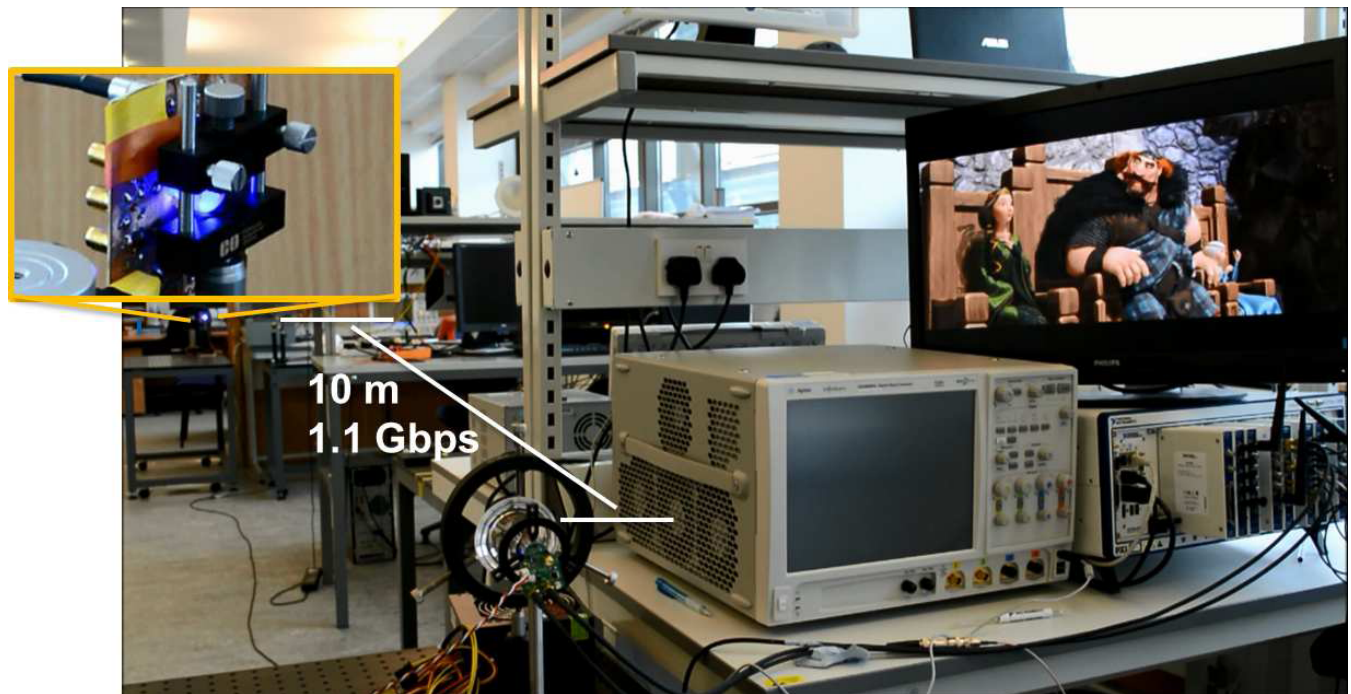
FIGURE 24. Demonstration of 1.1 Gbps VLC-aided video transmission system over a distance of 10m. The VLC transmitter is seen in magnified format at the top-left corner, which transmits the video signal to the receiver situated at the bottom of the picture. The received video picture is seen at the top-right corner.
