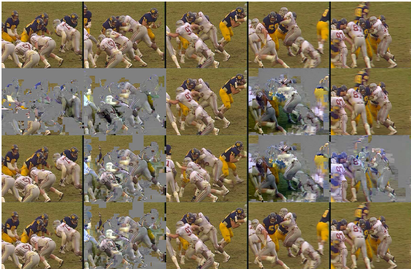
FIGURE 16. Five video frames of the ‘Football’ video test stream after video frame dropping, where the 4th, 8th, 12th, 16th and 20th video frames have been extracted from the original video stream (first row), UFR (second row), HFRFT (third row) and VT-2 (forth row) schemes, respectively. Observe with reference to the Fig. 15 that the UFR scheme imposes a PSNR degradation of 25 [dB] for the 4th video frame, which is similar to the HFRFT scheme, but a degradation of 0 [dB] is experienced to the VT-2 regime. Similar observation can be made at the remaining frame indices.
