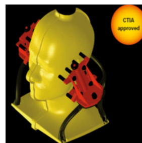
FIGURE A-1. SAM Phantom. “CTIA” is the Cellular Telecommunications Industry Association. Source: SPEAG Phantom Product Flyer.
