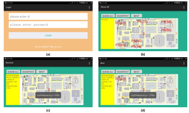
FIGURE 17. Implementation of the software system. (a) The login interface; (b) the map of all distributed car parks; (c) the result of the shortest case; (d) the result of our algorithm.
