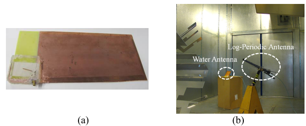
FIGURE 14. (a) Prototype of the water antenna, (b) RC set-up for antenna efficiency test.
