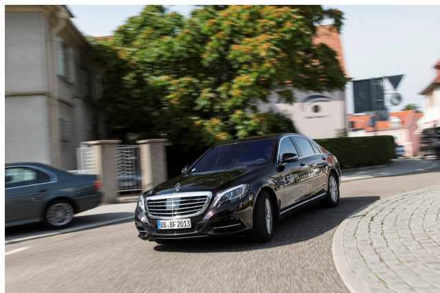
FIGURE 1. Autonomous vehicle “Bertha”, a 2014 Mercedes- Benz S-Class with well-integrated close-to-production sensors driving fully autonomously on open public roads.
