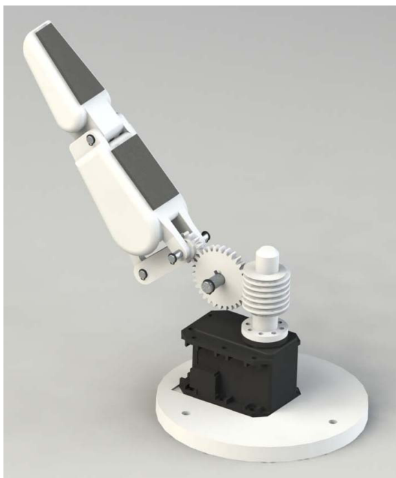
FIGURE 4. 2D (a) and 3D (b) sketches of the gear train design for one finger.
