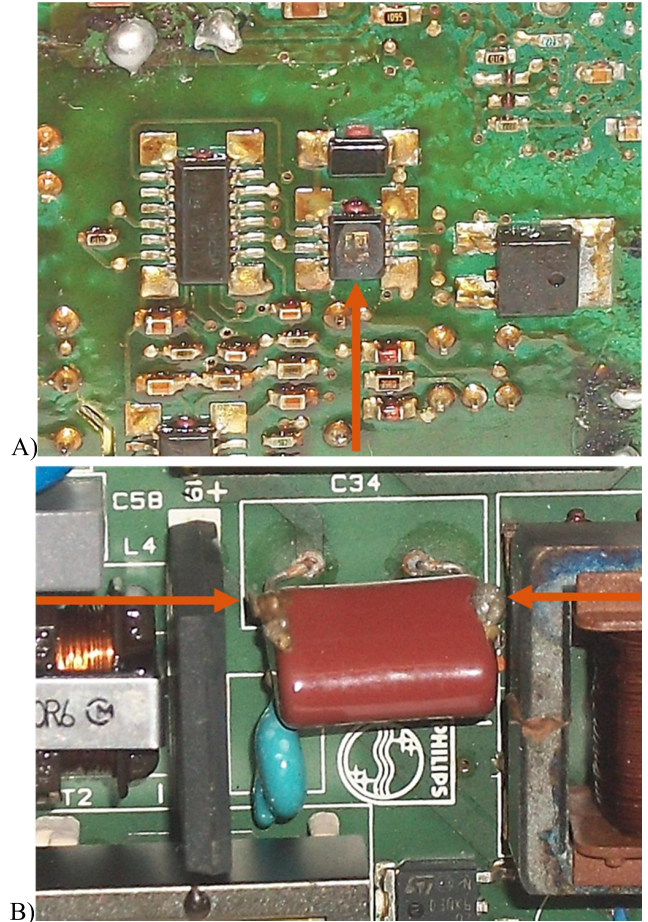
FIGURE 10. A failed A) IGBT/MOSFET and B) film capacitor inside the EDs. These predominate failure sites encompassed 70% of the EDs.
