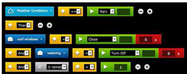
FIGURE 12. Twine (supermechanical.com) provides a user interface to define scenarios by combining sensors and actuators in a WHEN-THEN fashion which is also similar to the IF-THEN mechanism. Twine will trigger the actuation accordingly when conditions are met.
