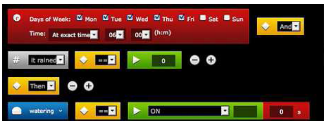
FIGURE 11. Two scenarios defined by using Fibaro (fibaro.com) platforms. The screen-shots show how different types of context triggers can be defined by combining sensors, actuators and predefined parameters.
