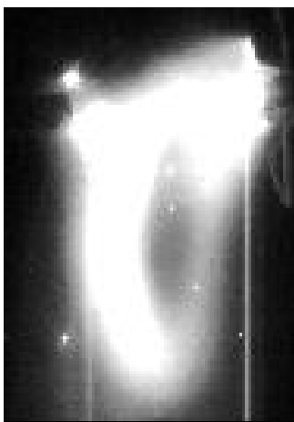
FIGURE 2. A 7.9 cm Electron Spiral Toroid Spheromak moving away from the initiating arc at the top of the image.
