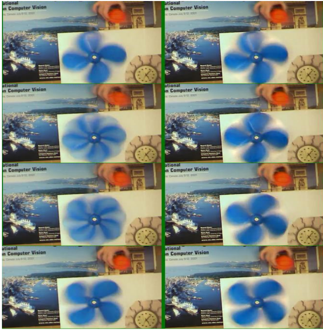
FIGURE 9: Comparison of Temporal Super-Resolution (3x): Bicubic Interpolation Method (Left) vs. Our Method (Right)
