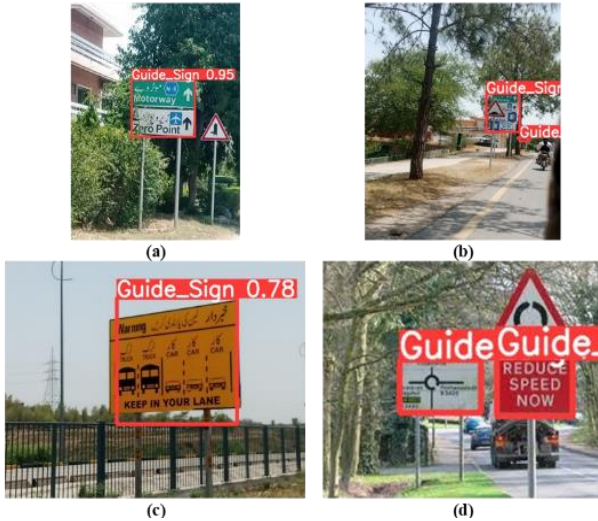
FIGURE 3. Traffic Panel Detection Using YOLOv5s in Images of Different Orientation and Resolutions: (a) and (b) Portrait Orientation and (c) and (d) Landscape Orientation
