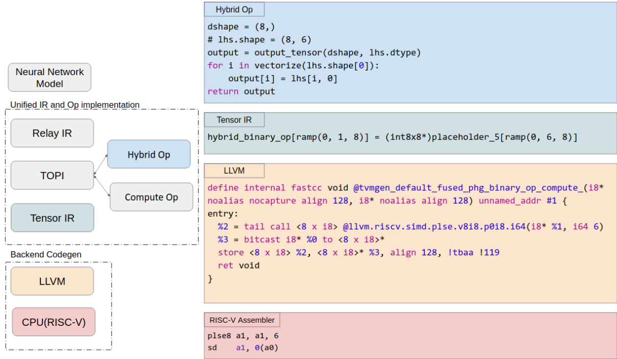
FIGURE 4. Enabling RISC-V custom instructions. We take PLSE8 as an example to show how we enable the transformation of custom instructions from TVM to RISC-V assembly language.
