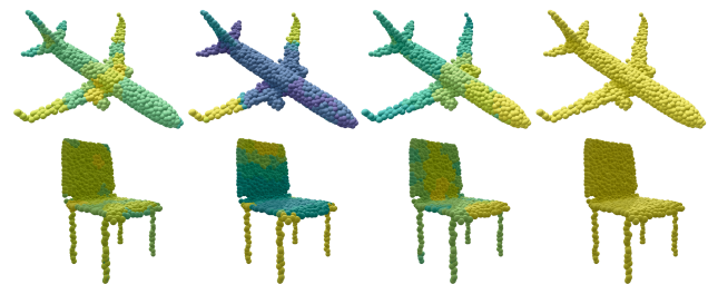
FIGURE 8. Attention scores of the classification token, averaged across all heads, pretrained using the MoCo pipeline. We visualize a subset of the network layers, [1, 3, 7, 8] left to right. While in the early layers the CLS token attends to meaningful parts of the shape, exhibiting a tendency to attend at symmetric parts, from layer 8 and onwards it attends uniformly to the whole shape.
