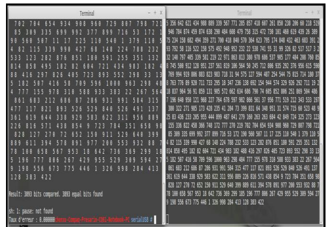
FIGURE 29. Program compilation chain BER test for wired link.
