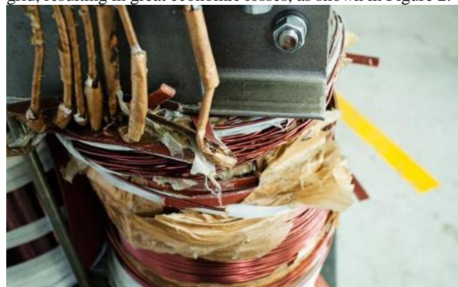
FIGURE 2. Insulation faults in power transformers.
