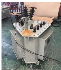
FIGURE 9. Arrangement of thermal resistance temperature measurement system.
