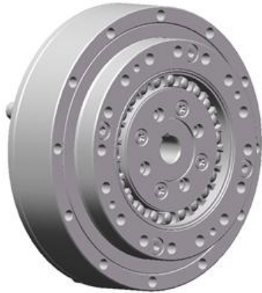
FIGURE 1. Harmonic reducer model diagram
