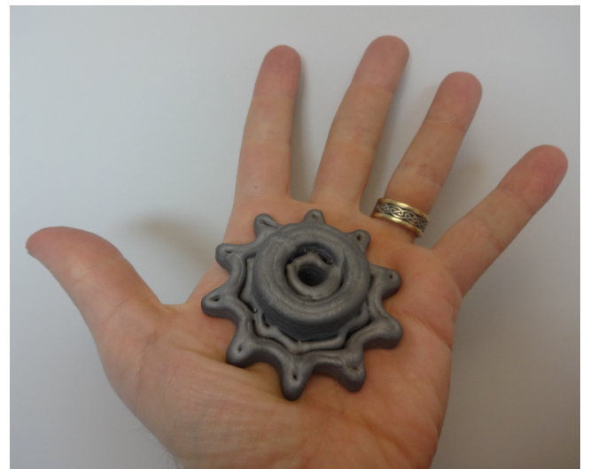
FIGURE 4. 3-D printed customized sprocket removed from the substrate.
