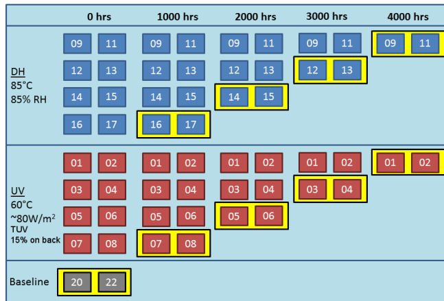
FIGURE 1. Modules harvested for each exposure condition (damp heat and UV preconditioning) showing the two modules removed at each time point. DH stands for damp heat, RH for relative humidity, and TUV for total UV.
