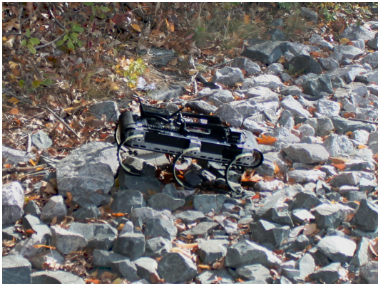
FIGURE 6. X-RHex performing a reactive stand on rocks.
