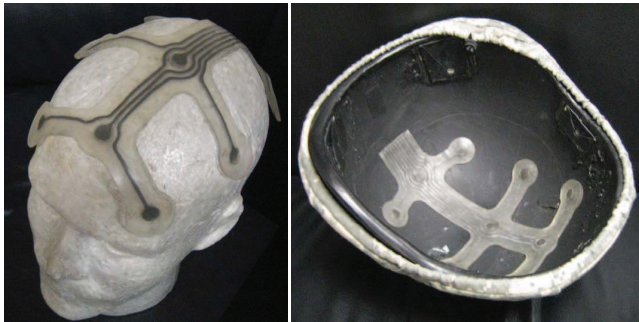
FIGURE 5. Stretchable, pliable conductors for biosensing. Example prototype 9-sensor strip of stretchable, pliable materials usable for EEG data collection can stretch beyond 33%. This technology allows it to easily conform for differing head sizes (left), while also providing comfort and safety of the user when built into head protection devices.
