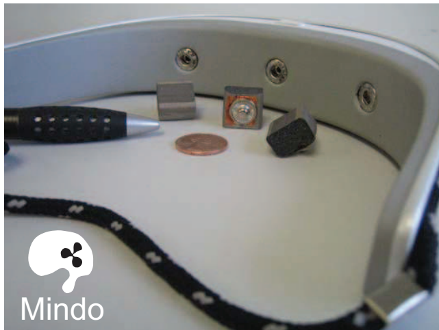
FIGURE 3. An early prototype system for BCITs. The NCTU-developed MINDO-4 system for potential BCITs that detect and mitigate fatigue-related performance decrements during driving. System uses soft pads (U.S. penny and pen shown for scale) that snap into a headband, and streams data via Bluetooth for easy system integration.
