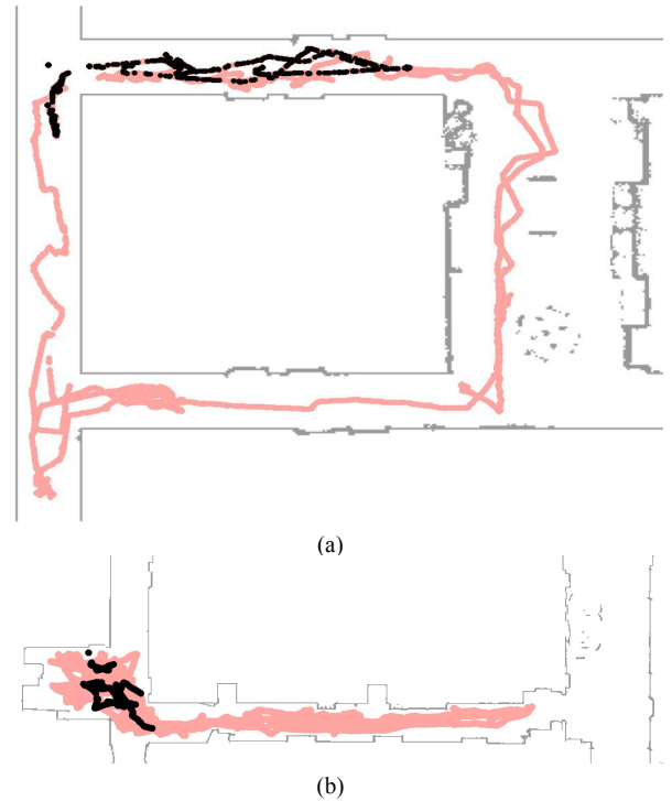
FIGURE 4. Local training locations. The local training set \mathbf{Y}_T is determined for (a) Levine and (b) Towne buildings by choosing 2% of the measurements in a subset of the environment—displayed here as black points.
