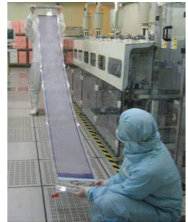
FIGURE 11. The R2R process flow of i2R (left) and finished e-paper measuring 3 meter long (right).
