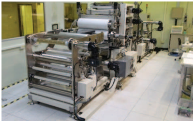
FIGURE 17. Photo of the R2R machine with dual functionality: (1) Incoming quality control in the far end, (2) Lamination in the near end of the photo.
