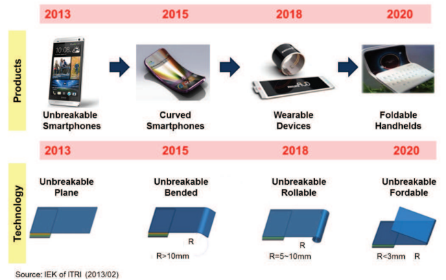
FIGURE 2. Progression in the development of flexible AMOLED technology and products.
