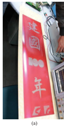
FIGURE 12. The passive matrix addressing (a) an e-banner and (b) an e-signage.
