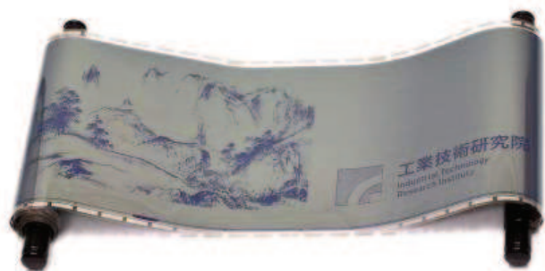
FIGURE 14. Demonstration of a Chinese landscape painting with the thermal addressing i2R e-paper.
