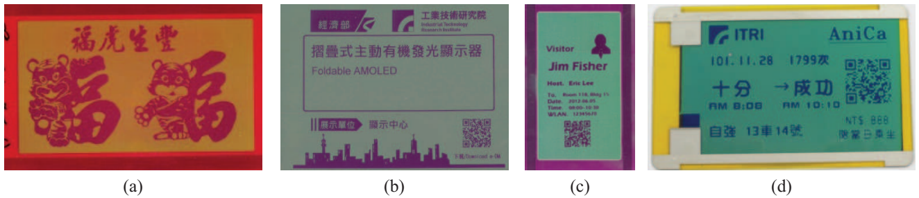
FIGURE 16. New applications of e-paper for (a) e-card (6 cm × 9 cm), (b) e-tag (13 cm × 16 cm), (c) e-badge (6 cm × 9 cm) and (d) e-ticket (5.4 cm × 8.5 cm).
