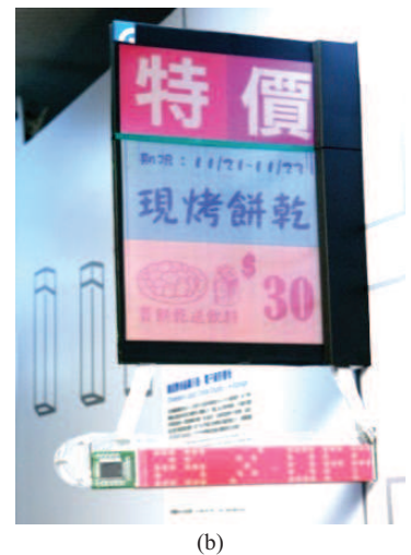
FIGURE 12. The passive matrix addressing (a) an e-banner and (b) an e-signage.
