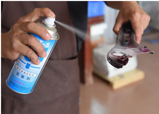
FIGURE 2. Developer spraying operation on parts using a device with its own high-pressure gas in a bottle.
