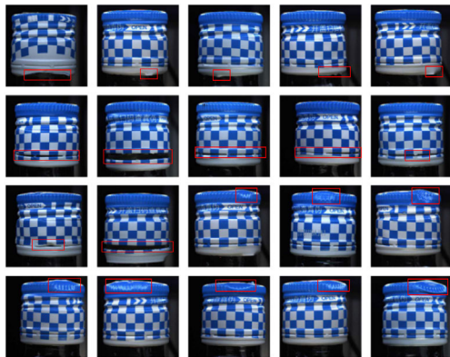
FIGURE 5. Example of a sample of Bottle-Cap. The figure contains anomalies such as deformation, dents, and crushing, and the anomalies are labeled with red boxes.
