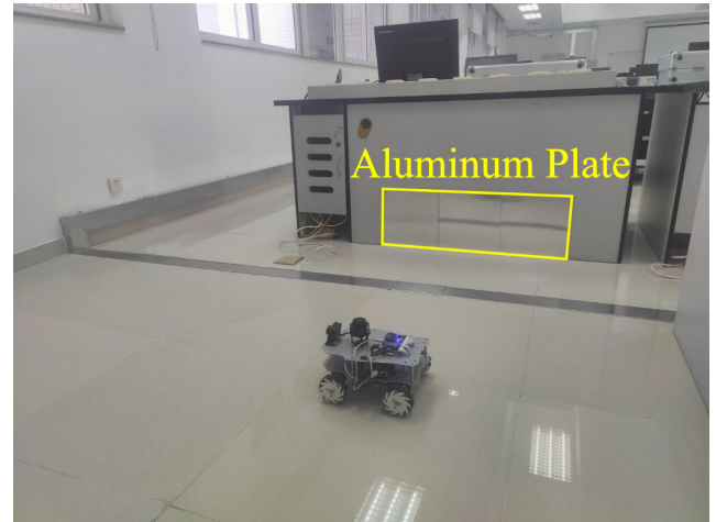
FIGURE 6. Scene setup for measuring the laser intensity value at the location of the aluminium metal plate.
