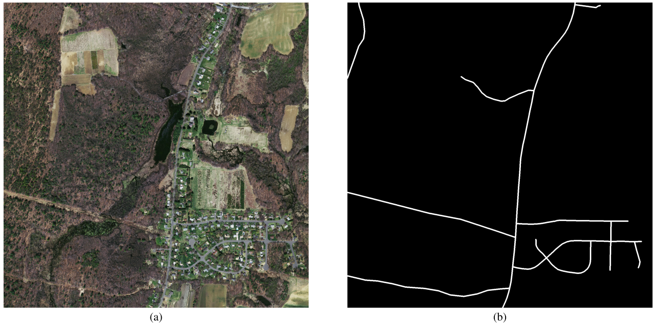
FIGURE 1. Example of (a) an aerial image and (b) the corresponding mask from the Massachusetts Roads Dataset [37].
