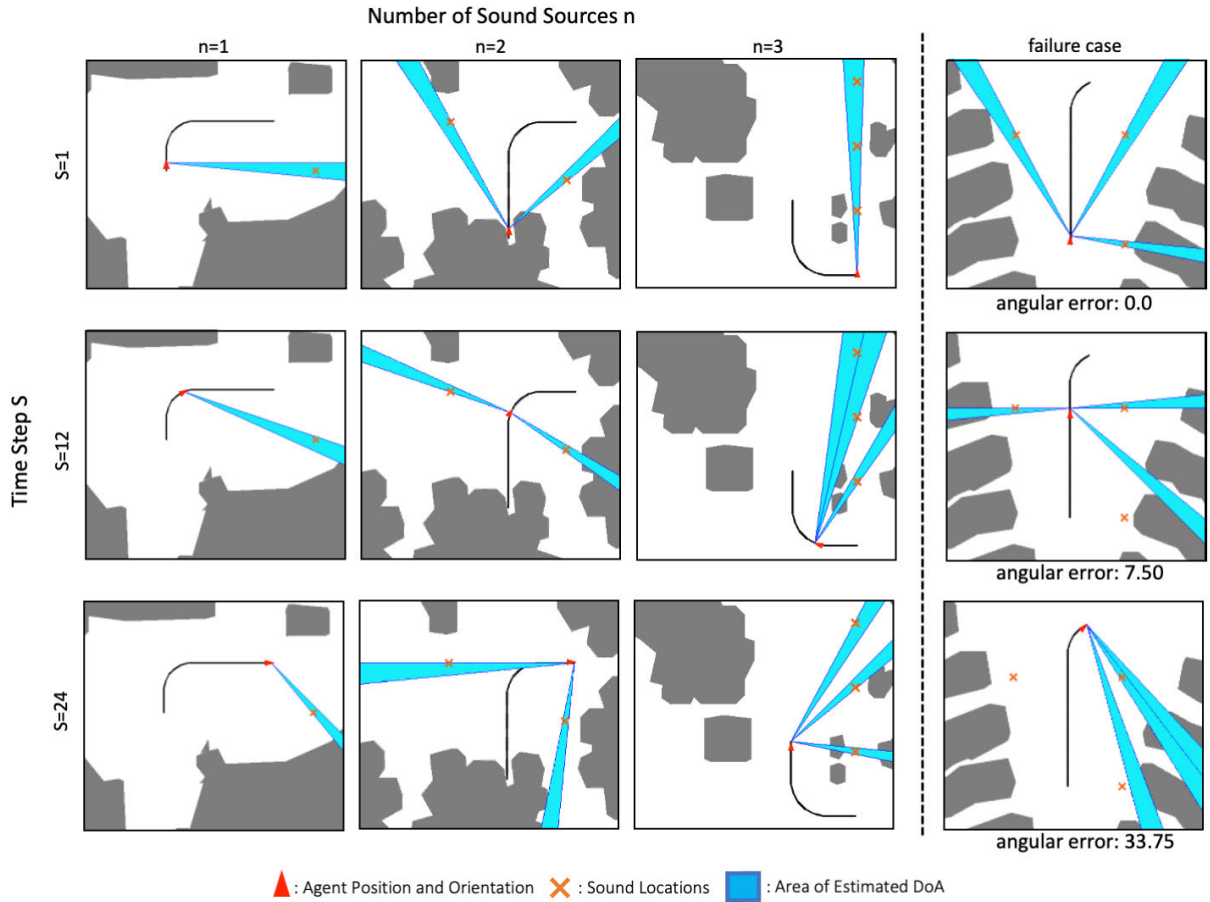
FIGURE 7. Visualization of DoA estimation using the proposed method. The three columns from the left are for 1, 2, and 3 sources, respectively. The rightmost column is the failure case.
