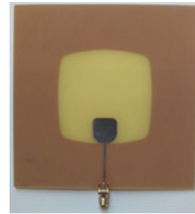
FIGURE 10. Geometry of optimized microstrip-fed supershaped wide-slot antenna.
