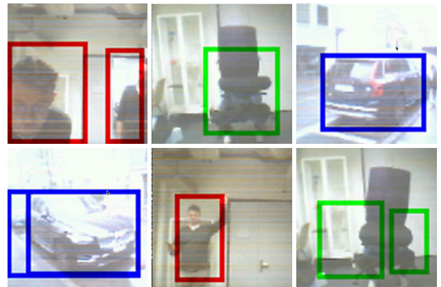
FIGURE 5. Example recordings of images with MAX78000 running an inference of TinyissimoYOLO on the recorded images.
