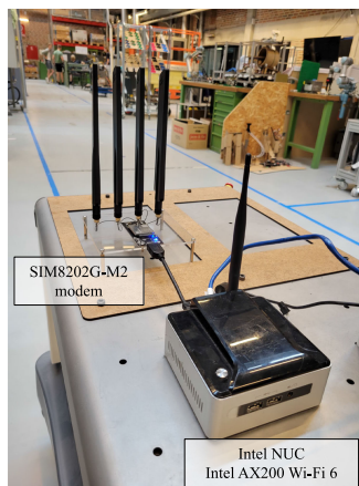
FIGURE 3. Picture of the equipment used to evaluate the network performance.
