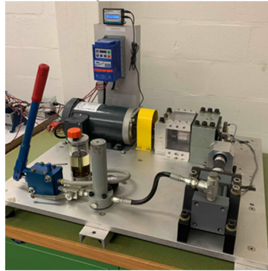
FIGURE 9. UNSW dataset test bench.
