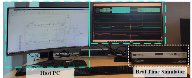
FIGURE 9. Experimental SIL test setup for real-time validation of the proposed DNN-based speed and current controller using OP-4510.
