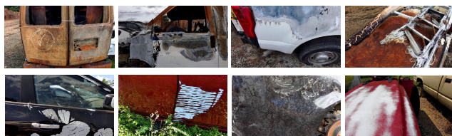
FIGURE 10. Samples of the defect categories that characterize intra-class defect similarities in the NCAT12-DET dataset. The first row depicts the different varying object instances of the burnt surface defect category. The second row depicts the background, occlusion, and viewpoint variation that characterize the defaced-paint defect category.
