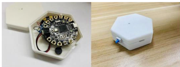
FIGURE 16. 3D printed prototype of the XR CUBE.
