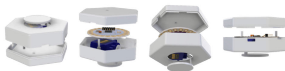
FIGURE 10. Acupressure sensation simulation device based on mechanical structure design.
