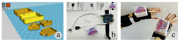
FIGURE 14. Wearable encapsulated boxes. a: model drawing of wearable encapsulated boxes; b: physical drawing of wearable encapsulated boxes; c: schematic diagram of the actual wearing of wearable encapsulated boxes.
