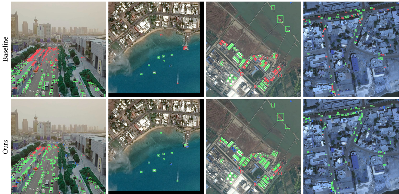
FIGURE 8. Visualization of sample test results on AI-TOD dataset, comparing the baseline detector (first row) with the AFS-based detector (second row). True positive (TP), false positive (FP), and false negative (FN) predictions are represented by green, blue, and red boxes in images, respectively.
