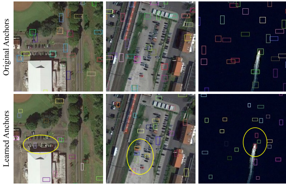
FIGURE 4. Stochastic visualization of original and learned anchors. The original anchor has strong regularity (first row), and the learned anchor is more flexible and can adapt to the tiny instance (second row). Notice that the visualization is performed on a small random portion of anchors for a clear view.
