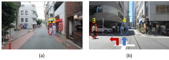
FIGURE 1. Overview of our work. As shown in the (a), which is easily understandable for human drivers, the significance of the first pedestrian outweighs that of the second, as humans recognize that pedestrian 1 is walking within the driving lane, whereas pedestrian 2 is not. Human drivers grasp an inherent relationship between pedestrians and line markings. As depicted in (b), even within the same intersection, the significance of objects can vary based on fluctuations in the driver's intention: if the driver intends to turn left, pedestrian 3 becomes the most important, whereas if the intention is to go straight, pedestrian 4 takes precedence.
