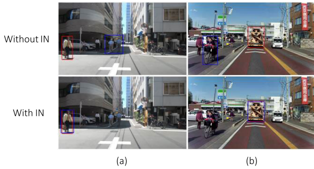
FIGURE 6. Visual ablation results for driving intention. IN represents the intention. The first column shows the IOL results of our method when excluding the driving intention module, while the second column displays the detection results of our model including the driving intention.
