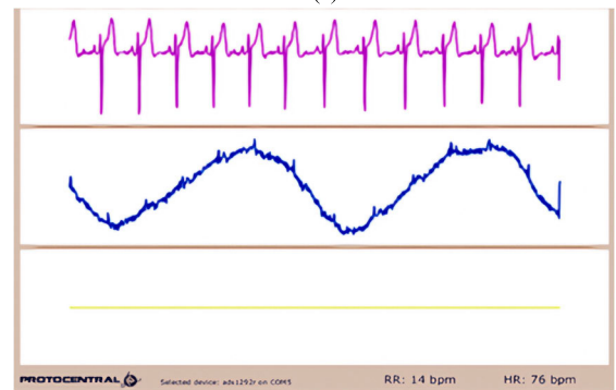
FIGURE 10. Feedback parameter measurement by hardware. (a) PPG signal with SpO 2 level 98.34% and (b) ECG signal and respiratory signal with RR & heart rate.
