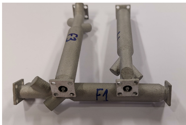
FIGURE 15. Photograph illustrating some manufactured prototypes without the coaxial connectors attached, showing the flange details at the connection face.
