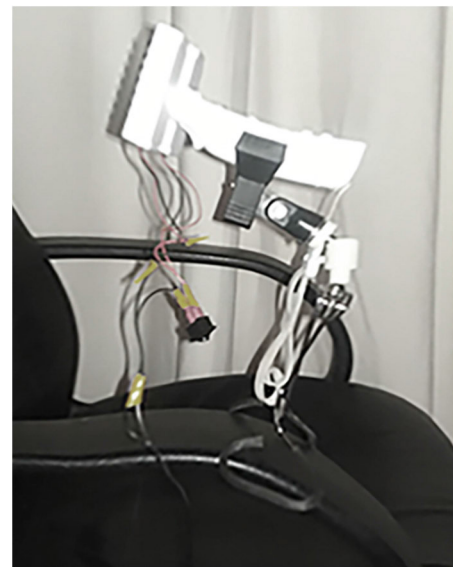
FIGURE 9. The complete TMIS shown as mounted to the chair handles with a clamp.
