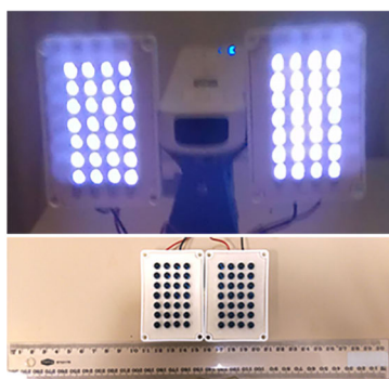
FIGURE 6. Final infrared array system and its dimensions: A close-up of the mounted system (above) and actual dimensions of the Infrared array; W = 100mm; H = 85mm, (below).
