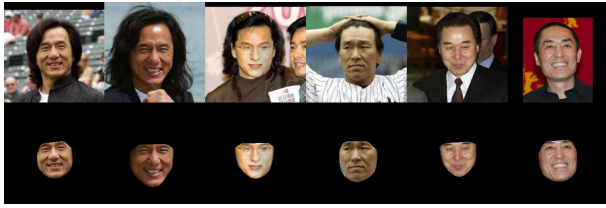
FIGURE 4. Example of human test questions. Row 1: unmasked question example. Row 2: masked question example. Column 1 shows the given examples; column 2 features the same individuals in a different frame; column 3 presents images on which our de-identification technology has been applied; columns 4-6 contain images deemed similar to the examples by FaceNet512.
