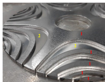
(c) The proposed BLR test module for a synchronous reluctance machine with 3 mm thick flux guides and 0.25 mm austenitic steel backplate. The d-axis flux guide forms a self-supported spider while the outer flux guides need to be fixed to the austenitic nonmagnetic steel backplate to maintain their positions. In this example case, the axial ferromagnetic material space factor of the rotor module is 92.3 %.
