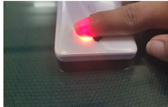
FIGURE 3. Video recording process: Finger is placed covering both camera and flashlight. A 1-minute video is recorded preferably from the index finger of the subject.
